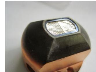
Metal (Al) filter ( $\sim \mu\text{m}$  thick window)
